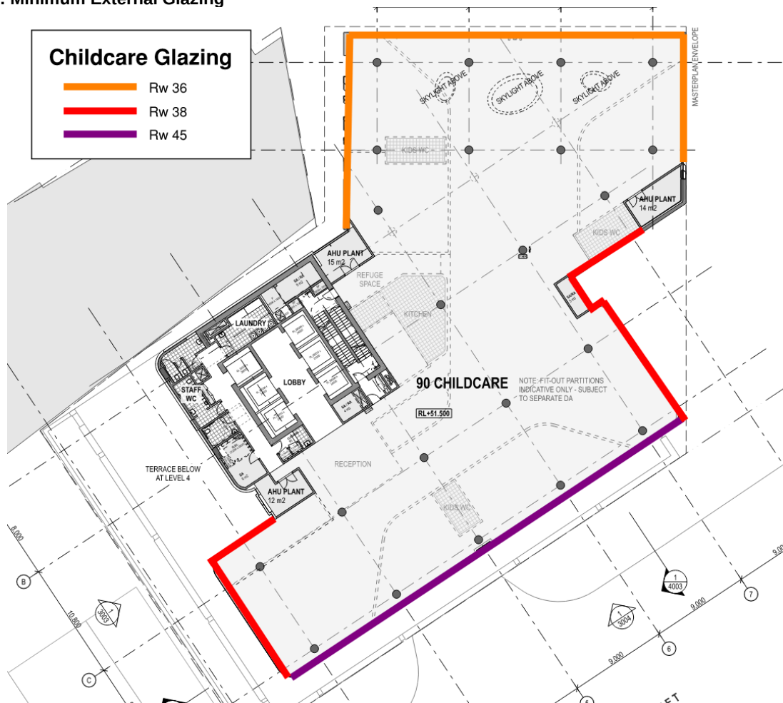
Figure 5: Minimum External Glazing
